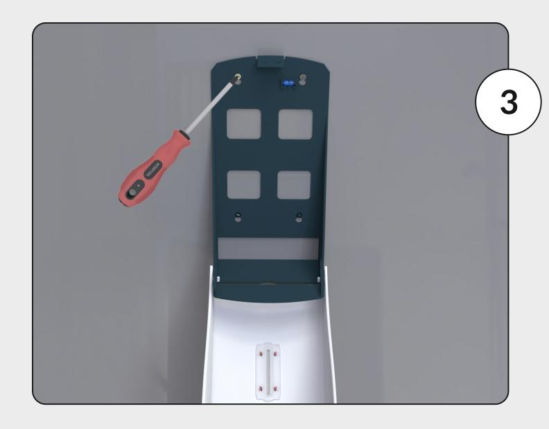
Drill the marked out holes to the size of the fixings provided then use a screwdriver to fix the unit to the wall. The unit should be hand tight to the wall.
