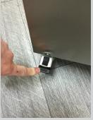
3. Push your machine to a suitable area and lock the brake lever to avoid the machine moving during use.
