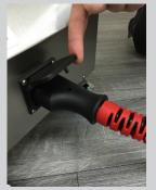
2. Lift the flap on the steam hose socket and connect the hose ensuring the pin locks into position.
