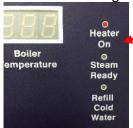
Allow approximately 5 minutes for the boiler to heat the water
