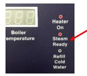
Re-allow the temperature to increase and the steam ready light will re illuminate (9)
