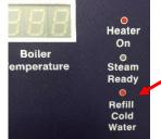
A buzzer will sound and the steam will no longer come out of the nozzle when the steam switch on the handle is pressed.
